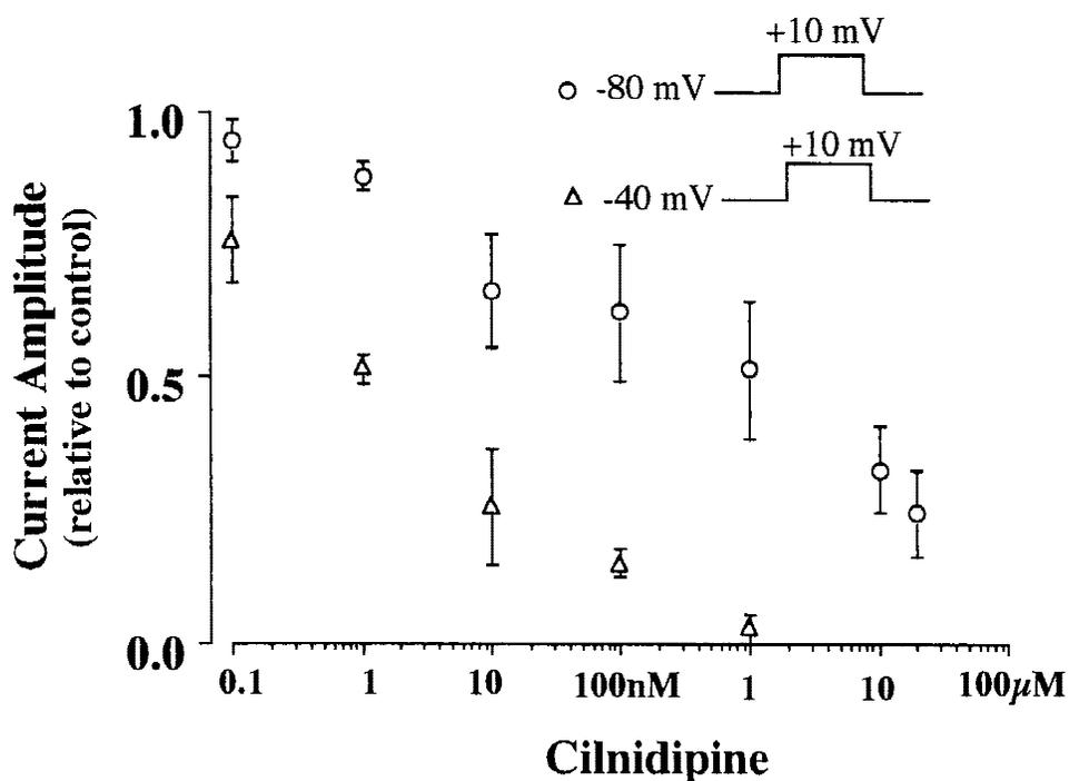
**FIG. 4.** Resting membrane potential-dependent effects of cilnidipine on vascular L-type  $\text{Ca}^{2+}$  channel currents. Single smooth muscle cells were isolated from rabbit basilar arteries, and L-type  $\text{Ca}^{2+}$  channel currents were monitored under voltage-clamped conditions. The  $\text{Ca}^{2+}$  channel current was induced at two  $V_H$  of  $-80$  mV and  $-40$  mV in the presence and absence of each concentration of cilnidipine. Data are from ref. 19.
